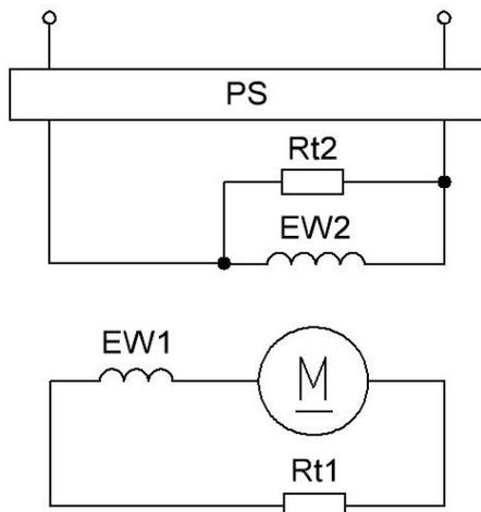
Fig. 2. Electric braking circuit using a mixed excitation electric motor
