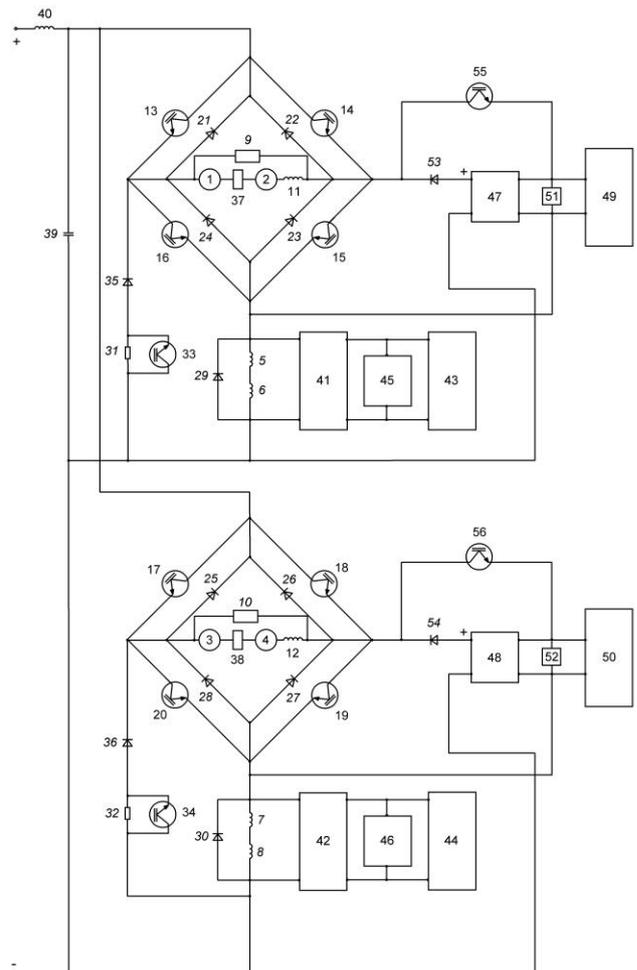
Fig. 5. Improved circuit design of electric braking system with variable structure
