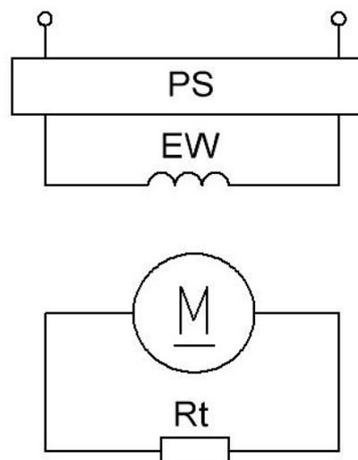
Fig. 1. Scheme of electrical braking during operation of the electric motor by an independent excitation generator
