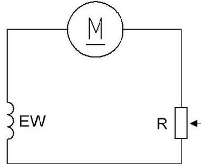
Fig. 3. Electric braking circuit when using an electric motor in the mode of a series excitation generator
