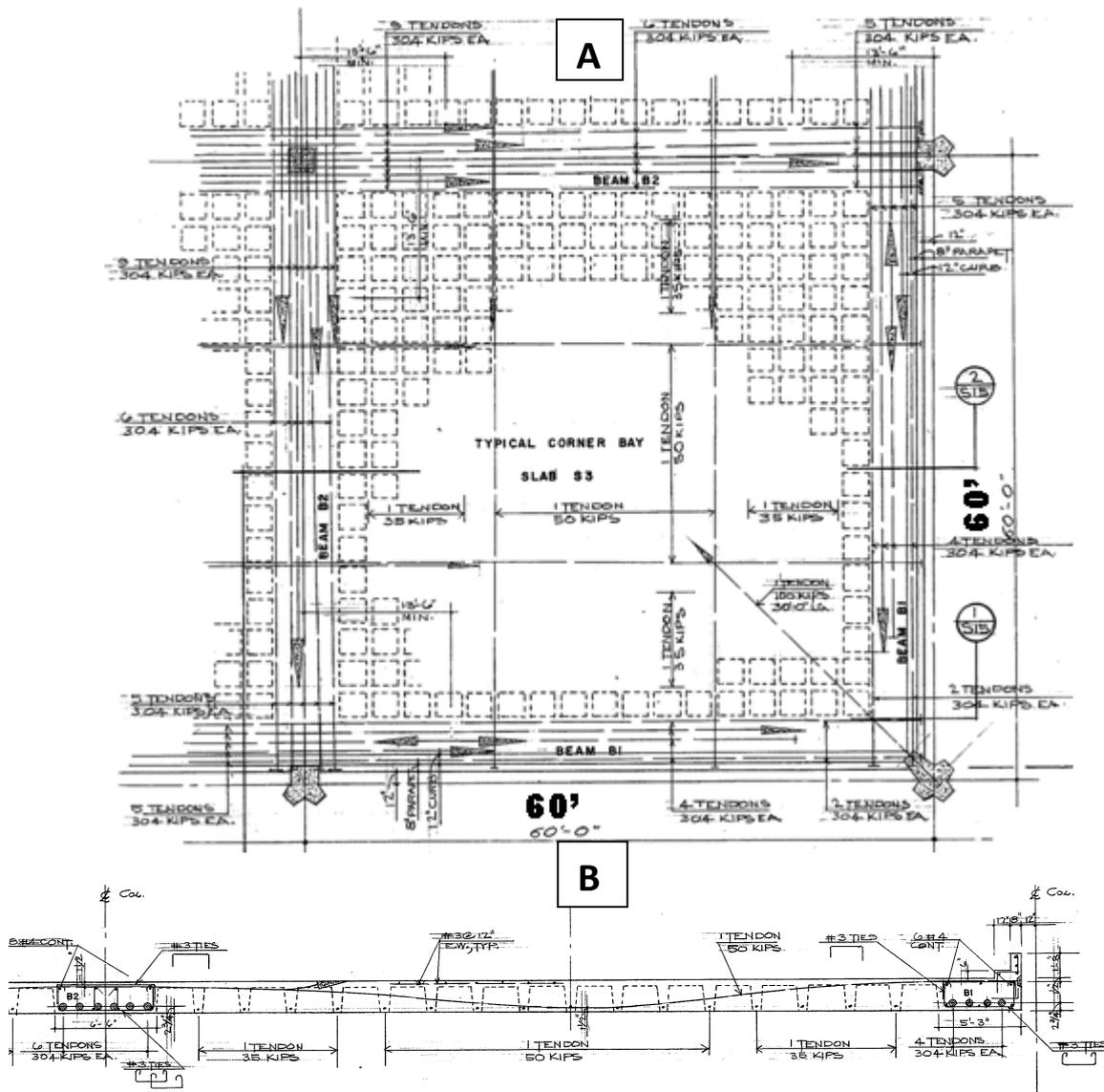
Fig.5. Plan (A) and Section (B) of a Corner Waffle Slab
