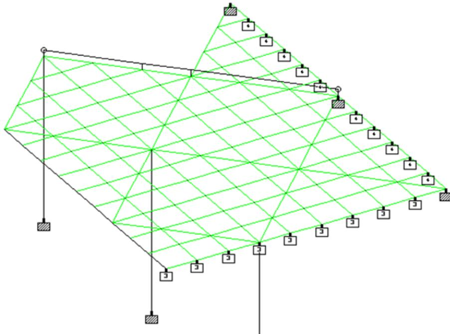
Fig.10. Model of Roof Corner after Cantilever Demolition for Analysis with Program STAAD.
